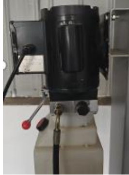
: Hydraulic hose connection to pump assembly.
